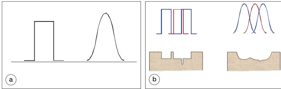
**FIGURE 73.4.** (a) Energy profiles of excimer laser beams. Top hat profile (left), Gaussian profile (right). (b) Adjacent spots produce the area of ablation on the cornea. Small displacements from the ideal spot location (middle spot) with top hat profiles produce more surface irregularity than is produced with Gauss profiles.
