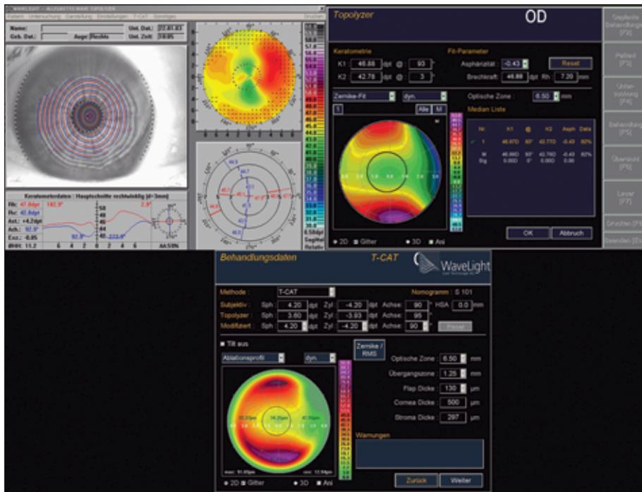
**FIGURE 73.8.** Topography of a cornea with irregular hyperopic astigmatism and corresponding differential elevation map. This map of the differences between measured and desired aspheric shapes of the cornea is converted into an ablation pattern.
