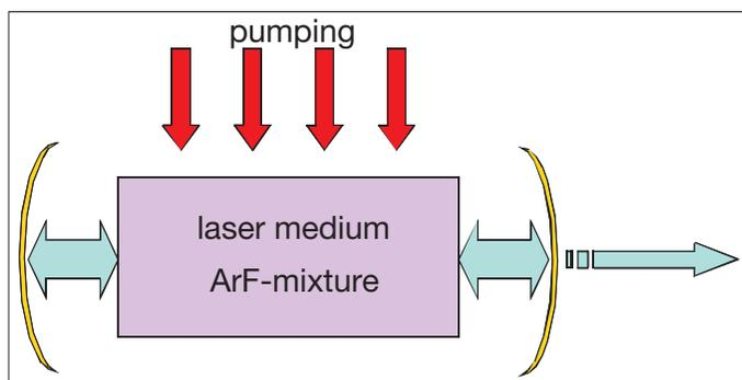
FIGURE 73.3. Schematic representation of a laser. In the case of the 193 nm excimer laser, the laser medium consists of a gas mixture and pumping is performed by means of an electrical discharge.
