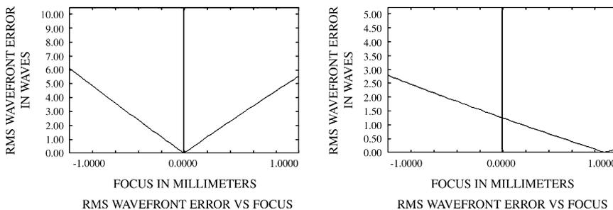
**Figure 2.** The RMS wavefront error as a function of the position in front of and behind the retina in the emmetropic nonaccommodated eye. The focus in the far distance configuration is located in the retina (left); in the near configuration it is shifted  $900 \mu\text{m}$  behind the retina (right).
