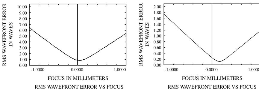
**Figure 4.** The RMS wavefront error as a function of the position near the retina with a CSI 3.0 mm in diameter and an additional refractive corneal power of 3.00 D. The image plane for near vision (*right*) is closer to the retina level than the GO, with the advantage of a better near vision and the disadvantage of no chance of improvement with glasses.
