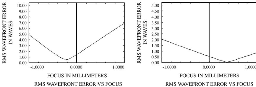
**Figure 3.** The RMS wavefront error as a function of the position near the retina with the GO regarding R and Q. Compared to the emmetropic eye, the wavefront error for far distance vision (*left*) has increased; however, in the near configuration, the focus (*right*) is located only 400  $\mu\text{m}$  behind the retina and may be shifted into the retina level by means of reading glasses.
